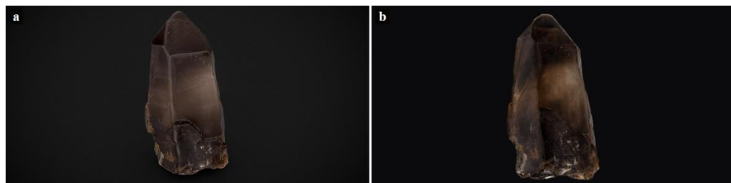
Fig. 1 The same smoky quartz specimen as a) a photogrammetric textured mesh (Sketchfab) and b) a 3D Gaussian Splatting model, which preserves its translucency, colour zoning and inclusions (Apopei, 2025b).
